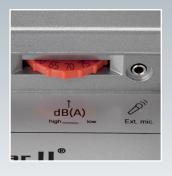
Use the red wheel at the bottom of SoundEar II to set your noise limits. SoundEar II provide a visual warning sign consisting of a flashing red light at 16 different noise limits ranging from 40 to 115 dB(A). Our website contains information on suitable noise limits.
