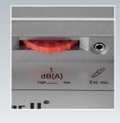
Use the red wheel at the bottom of SoundEar II to set your noise limits. SoundEar II provide a visual warning sign consisting of a flashing red light at 16 different noise limits ranging from 40 to 115 dB(A). Our website contains information on suitable noise limits.
